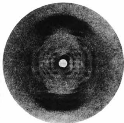
Fig. 5. Single fibre, about 40\ \mu diameter. Specimen-film distance 15 mm.; r.h. 75%; exposure about 100 hr. Photograph showing double orientation.
